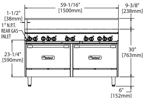
All 115V, 60Hz, 1 phase GFE models are supplied with a 6' (1829mm) cord and plug (NEMA-5-15P), 240V 50/60 Hz. 1 phase, 1.8 amps are not supplied with cord and plug and must be direct connect. Convection oven models draw 3.5 amps, standard GFE models draw 0.2 amps for the ignition system; 240V systems without the convection motor are 0.1 amps.
